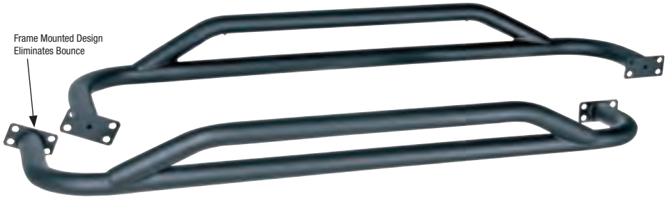
11504.11 RRC Rock Slider, Textured Black, 87-06 Wrangler
