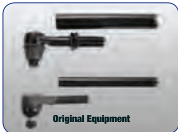
Rugged Ridge Heavy-Duty Tie Rods compared to Original Equipment
