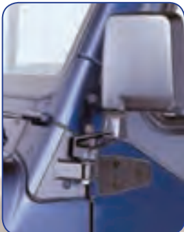
11025.02 Mirror Relocation Bracket, 97-02 Wrangler
