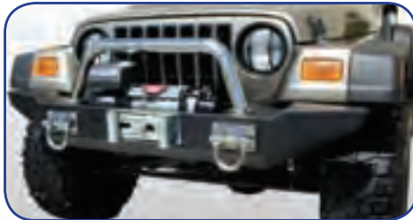
Standard Front Winch Mount With Stainless D-rings & Stainless Overrider Hoop: 11540.40, 11540.16, 11540.17, 11540.42
